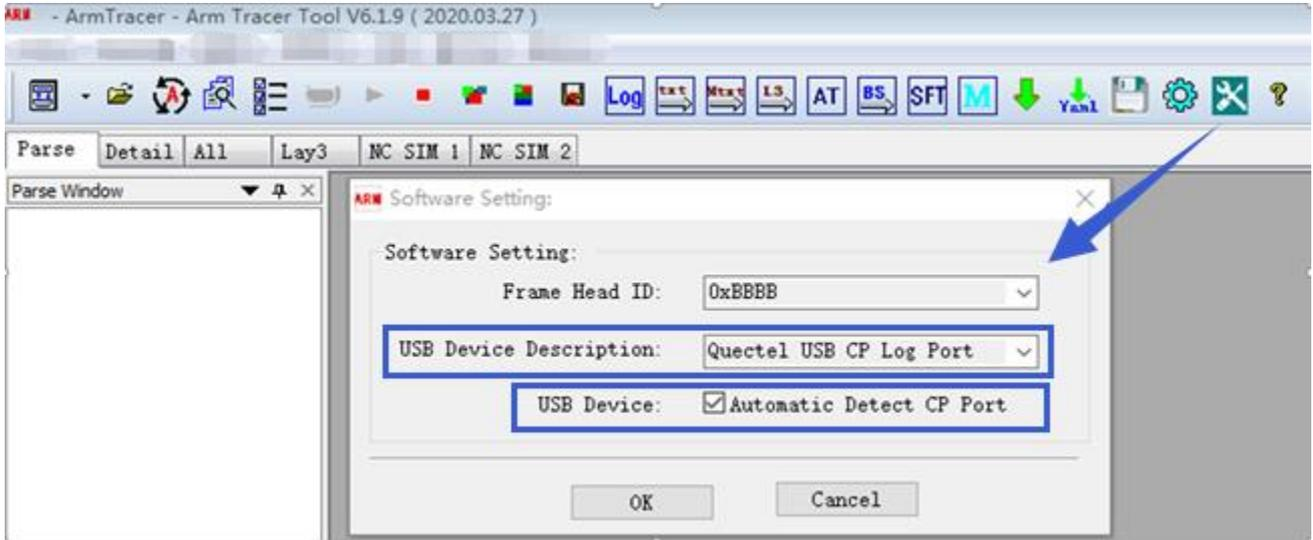
**Figure 12: Automatic Detect CP Port**
